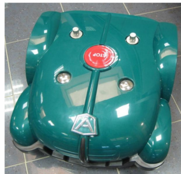
Picture 2 - New L200R robot cover with EMERGENCY STOP button
